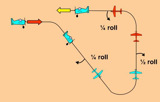
From upright, push through a one eighth loop into a forty-five degree downline, perform a quarter roll, perform a three eighths knife-edge loop into a vertical upline, perform a half roll, perform a quarter knife-edge loop, perform a quarter roll, exit upright.
