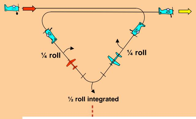
From upright, fly past center, push through a three eighths loop into a forty-five degree downline, perform a quarter roll, perform a quarter knife-edge loop into a forty-five degree upline, while integrating a half roll, perform a quarter roll, push through a three eighths loop, exit upright.
