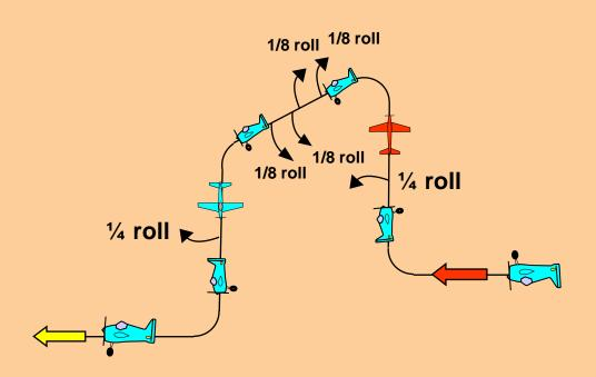
From inverted, push through a quarter loop into a vertical upline, perform a quarter roll, push through a quarter loop into a horizontal crossbox line, perform consecutively two one eighth rolls, followed by two consecutive one eighth rolls in opposite direction, push through a quarter loop into a vertical downline, perform a quarter roll, pull through a quarter loop, exit upright.
