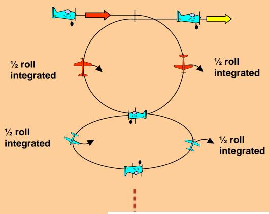
From upright, push through a half loop, while integrating a half roll, perform a crossbox circle with two half rolls in opposite directions integrated, pull through a half loop, while integrating a half roll in opposite direction of the half roll in the first half loop, exit upright.
