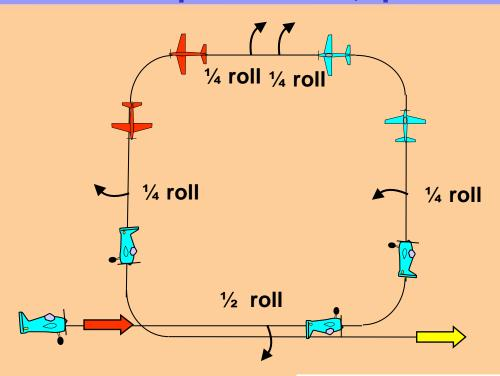
From upright, perform a half roll in the center, push through a quarter loop into a vertical upline, perform a quarter roll, perform a quarter knife-edge loop into knife-edge flight, perform consecutively two consecutive quarter rolls in the center, perform a quarter knife-edge loop into a vertical downline, perform a quarter roll, pull through a quarter loop, exit upright.
