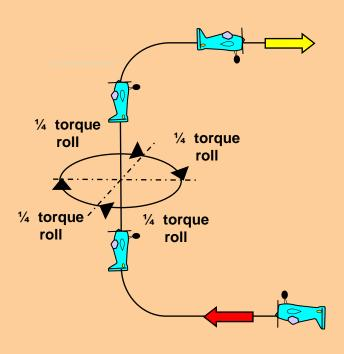
From inverted, push through a quarter loop into a vertical upline, perform consecutively four one quarter torque rolls on same level, push through a quarter loop, exit upright.
