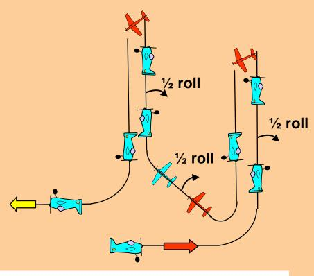
From upright, pull through a quarter loop into a vertical upline, perform a half roll, perform a stall turn into a vertical downline, perform a quarter knife-edge loop into a knife-edge crossbox line, perform a half roll, perform a quarter knife-edge loop into a vertical upline, perform a half roll, perform a stall turn into a vertical downline, push through a quarter loop, exit inverted.
