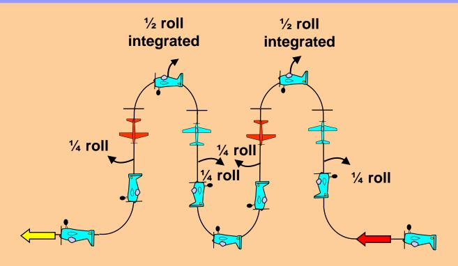
From inverted, before the center push through a quarter loop into a vertical upline, perform a quarter roll, perform a half knife-edge loop (towards the center) with integrated half roll into a vertical downline, perform a quarter roll, push through a half loop in the center into a vertical upline, perform a quarter roll, perform a half knife-edge loop (away from the center) with integrated half roll into a vertical downline, perform a quarter roll, push through a quarter loop, exit inverted.
